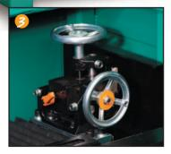
Vertical And Horizontal Adjuster when used for aligning with the digital gauge it produces the highest quality grind possible. This adjuster can also be used with the pushbutton infeed to "touch-off," if desired by the operator.
