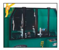
Electrically Interlocked Guardingsafety is ensured with doors that keep the operator and others from inadvertently entering the grinding "work" area.
