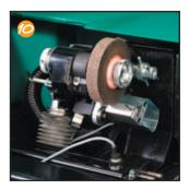
Grinding Head And Patented Relief Assembly-heavy-duty, dependable, rugged tool-type design that provides accuracy and fast spin and relief grind cycles.
