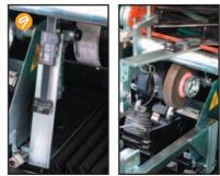
Digital Alignment Gauge-provides easy and accurate setup of the reel, ensuring that it is ground to a true cylinder, removing any "cone-shape" that typically develops in the cutting process.
