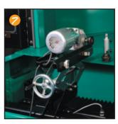
Spin Drive Unit—variable speed, reversible, and easy setup accommodates different reel configurations.
