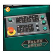
Control Panel-standard manual control is easy to operate due to the logical grouping of controls.
