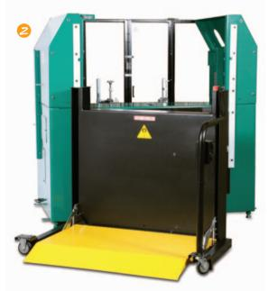
**Optional Workstation**—The NEW Workstation is used as a workbench in the maintenance shop, but can also be used to transfer reels into a grinding machine. Once transfer is made, The Workstation can easily be put into a stored position.
