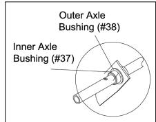
Note: Insert the Inner axle bushing into the outer axle bushing and make sure they are tight.
