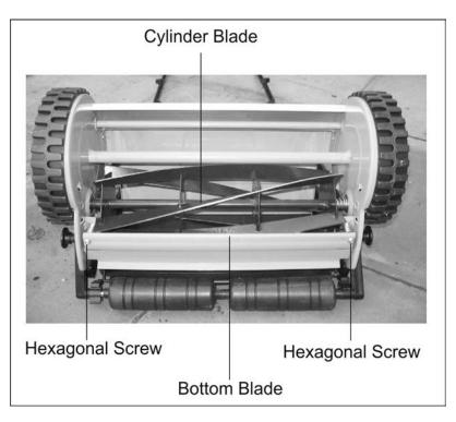
1. The hexagonal screws on the bottom blade assembly allow the distance from the cylinder and the bottom blade to be adjusted.
