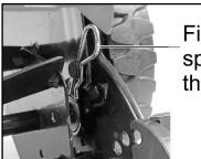
Fit the split pin to secure the handle Fit the Split Pin
